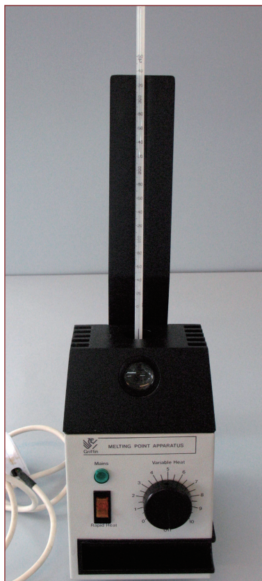
Figure 2.6 An electrical melting-point apparatus.
